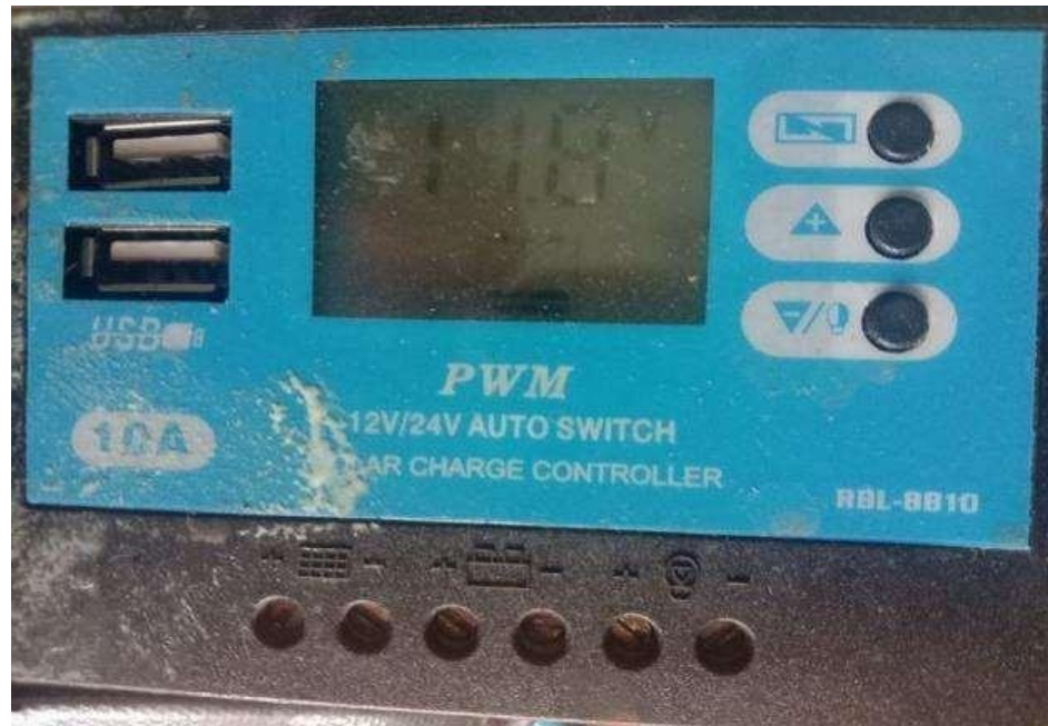
Gambar 3.3 Sollar Charger Controller
