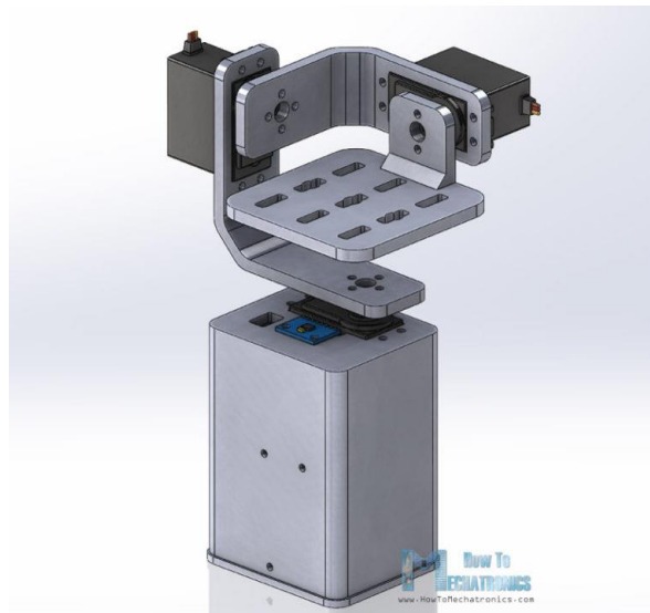
Gambar 3.2 Desain Gimbal Kamera Sumber: ( https://howtomechatronics.com )
