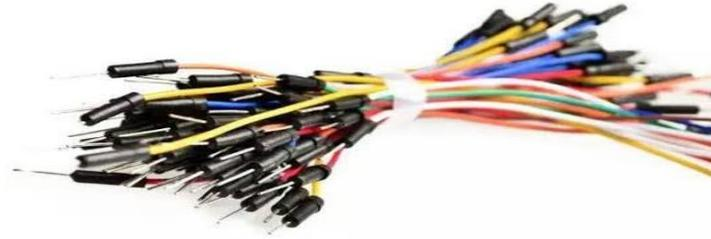
**Gambar 2.12 Kabel Jamper**
