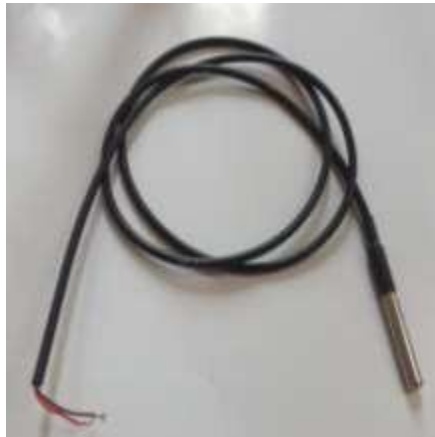
Gambar 2.3 Sensor suhu DS18B20
