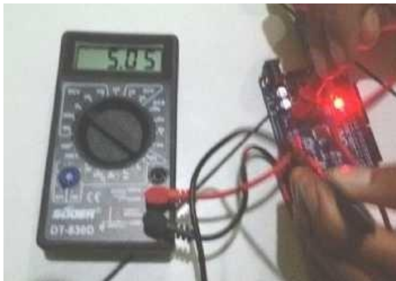
Gambar 4. 1 Pengujian Pin-pin Arduino Uno
