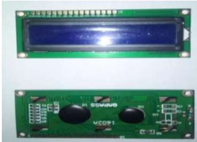
Gambar 2.7 Liquid Cristal Display (LCD)
