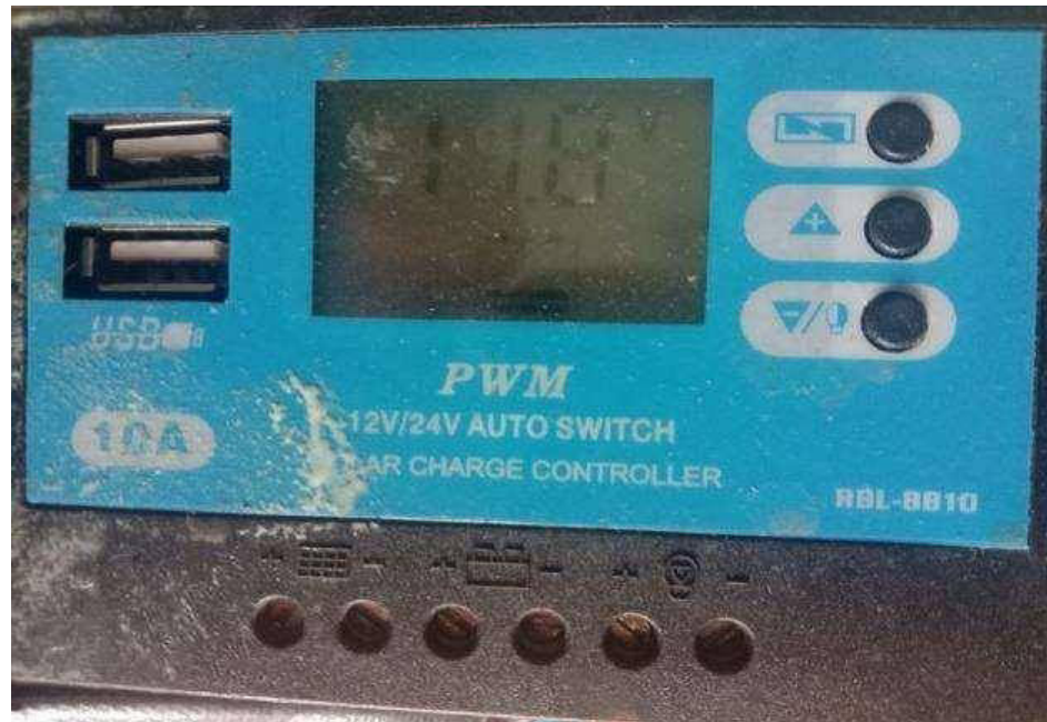
Gambar 3.3 Sollar Charger Controller
