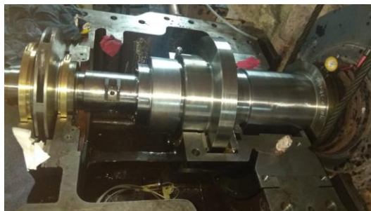
Gambar 2.16 Penggantian Thrust Bearing Team Mechanical
