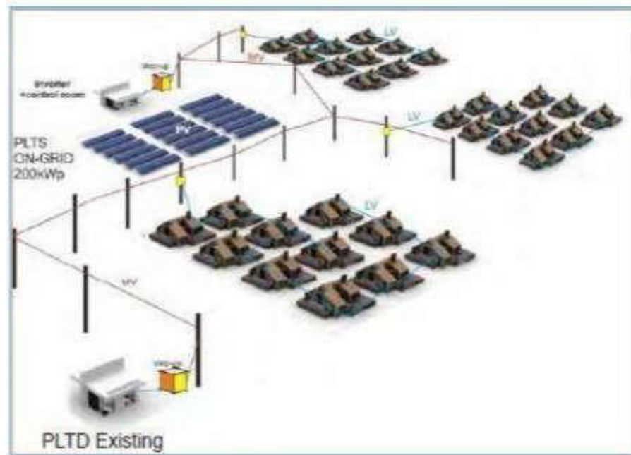
Gambar 2.4 Skema hybrid photovoltaic power system Roihan Abdullah,dkk 2018
