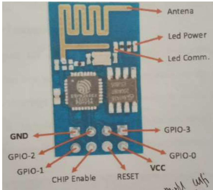
**Gambar 2.6 Modul ESP8266**
