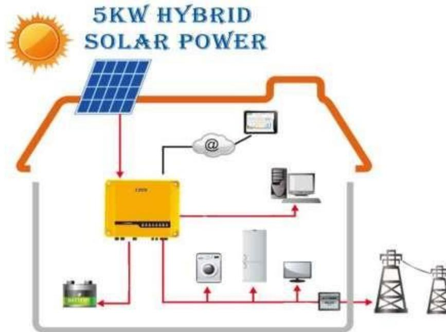
**Gambar 2.3 Prinsip Kerja PLTS On-Grid**
