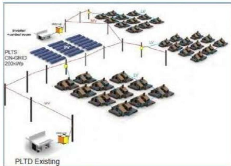
**Gambar 2.4 Skema *hybrid photovoltaic power system***
