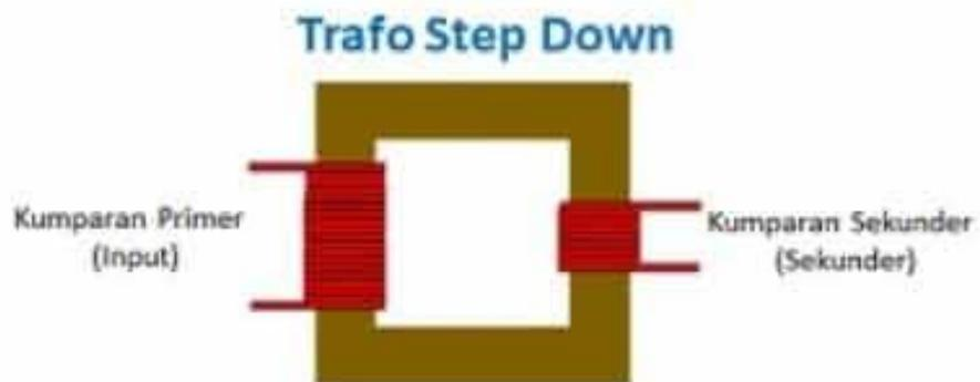
**Gambar 2. 3 Skema Trafo Step Down**
