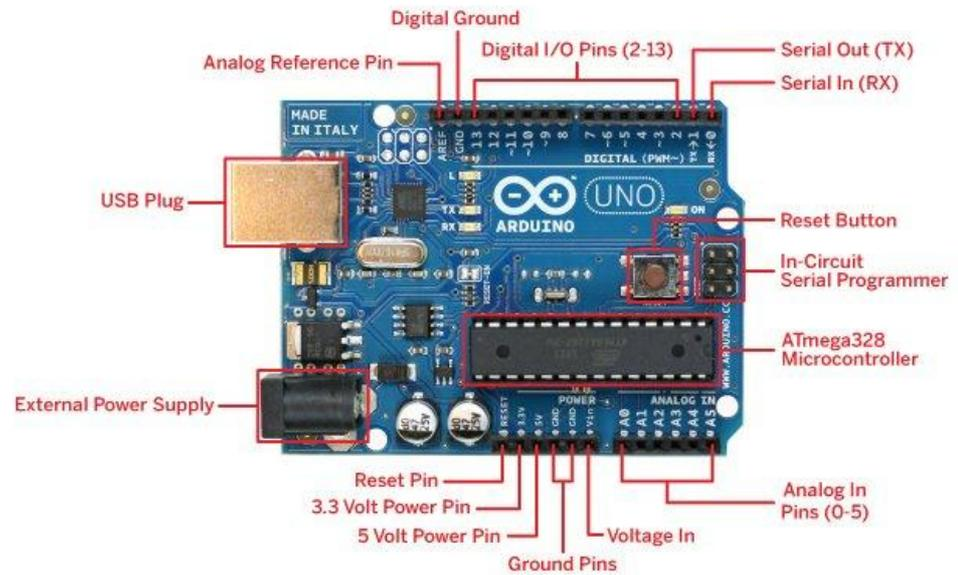
**Gambar 2. 8 Board Arduino Uno**
