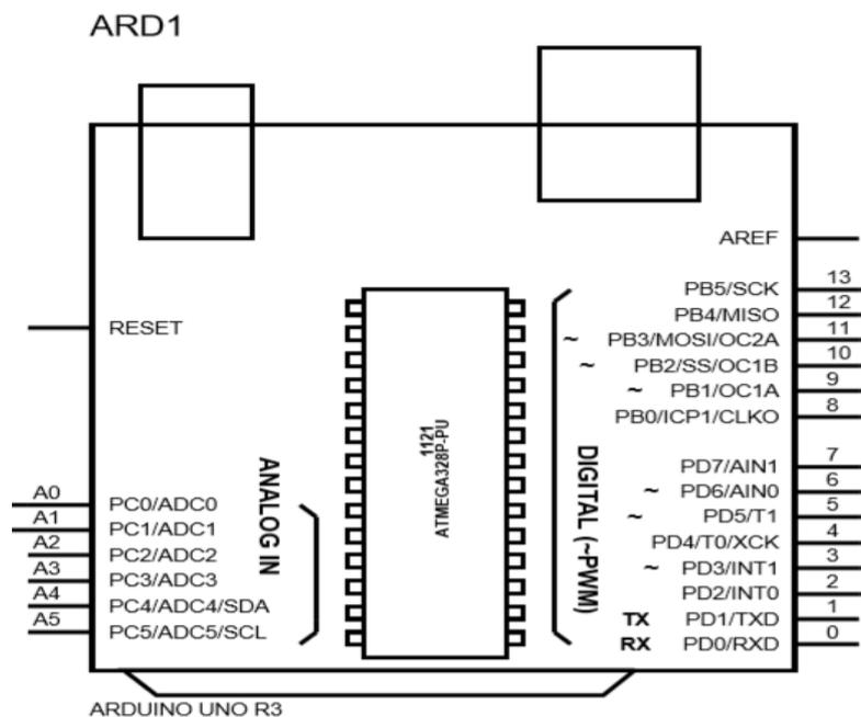
**Gambar 3.3 Port Arduino Uno**
