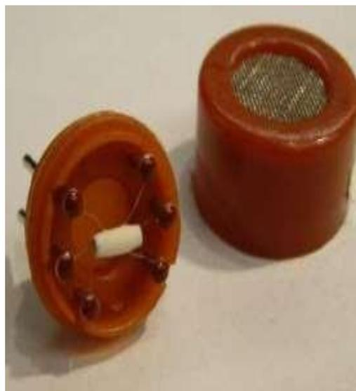
**Gambar 2.6** Internal Sensor MQ-2
