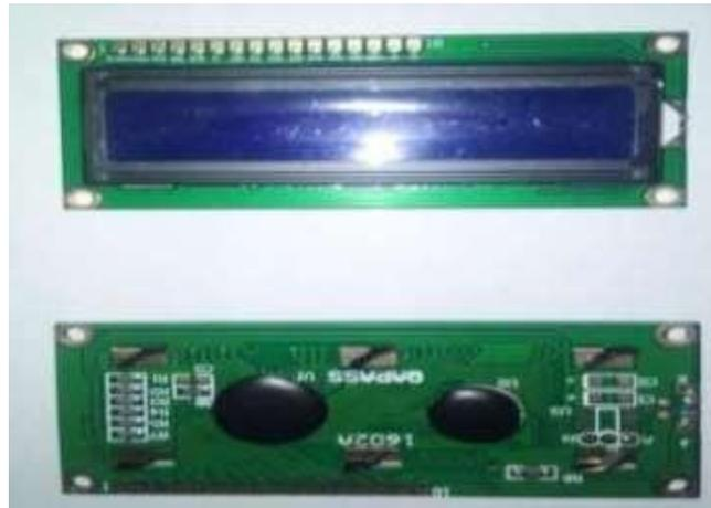
**Gambar 2.11** *Liquid Cristal Display (LCD)*
