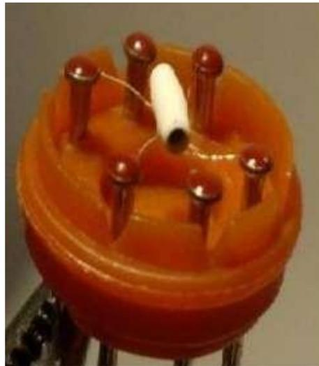
**Gambar 2.8** Prinsip Kerja Sensor MQ-2
