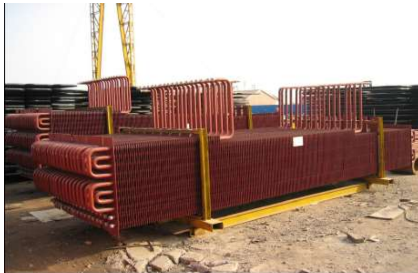
Gambar 2.12 Economiser Fineed Tubes (Tipe Pipa Bersirip) Sumber: PLN Corporate University, 2018
