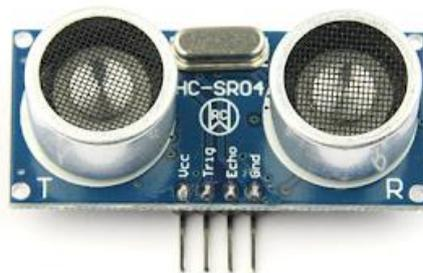
**Gambar 2.8 Sensor Ultrasonik HC-SR04**
