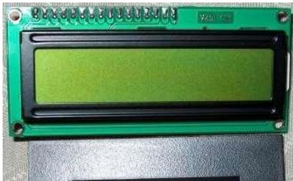
**Gambar 2.17 LCD 2x16**
