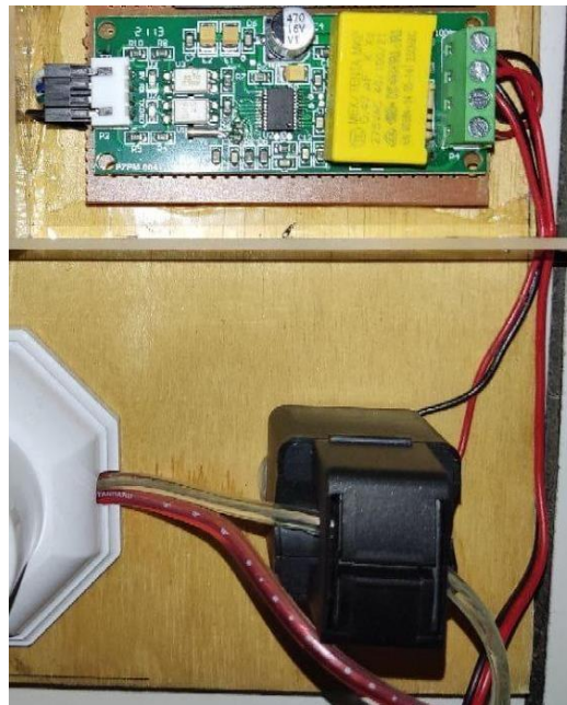
Gambar 4.4 Implementasi Sensor Arus PZEM 004T
