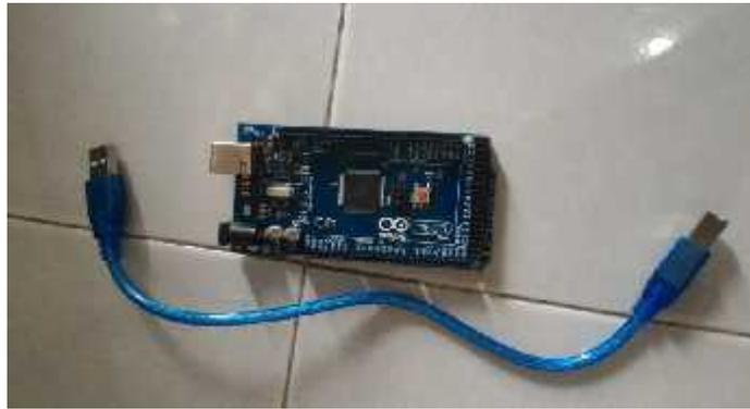
**Gambar 2.3 Arduino Mega 2560**
