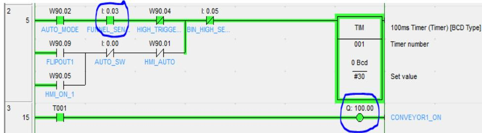
**Gambar 4.7 Ladder Diagram Mesin Conveyor ON**
