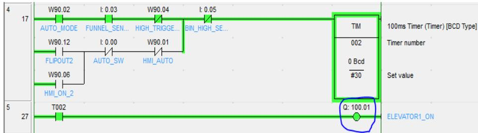
**Gambar 4.8 Ladder Diagram Mesin Elevator ON**
