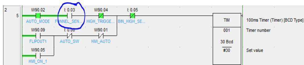
**Gambar 4.6 Ladder Diagram Sensor Intake**
