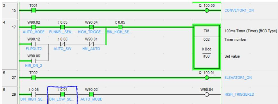
**Gambar 4.9 Ladder Diagram Low Level ON**
