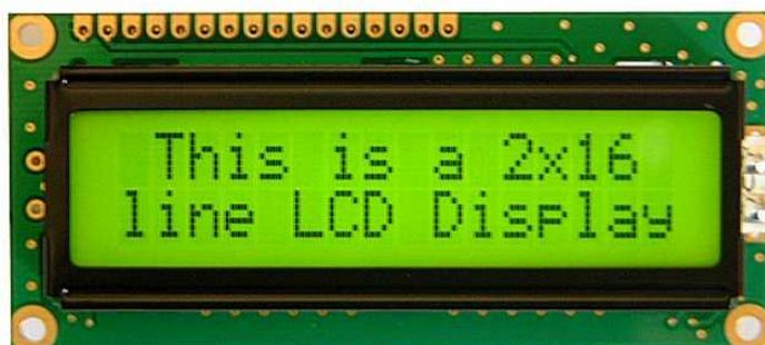
**Gambar 2.13.** LCD (*Liquid Cristal Display*)
