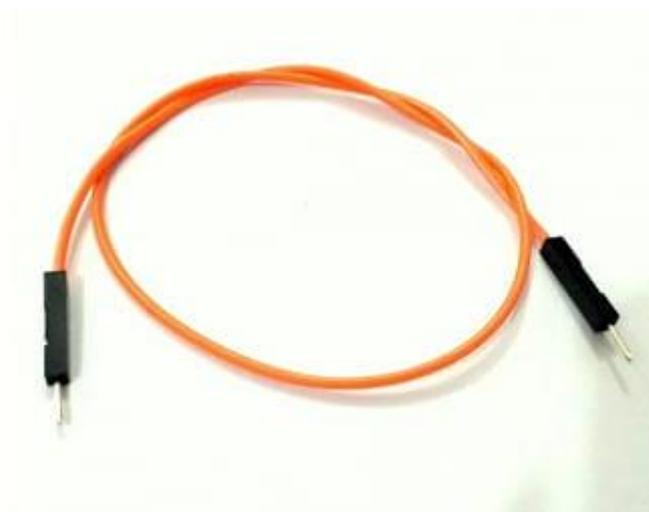
**Gambar 2.15** Kabel Jumper Male to Male
