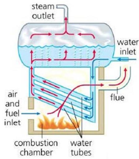
**Gambar 2. 6 Water Tube Boiler**
