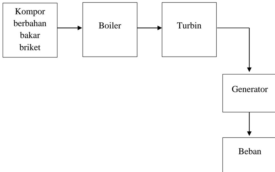
**Gambar 3. 1 Blok Diagram PLTU**
