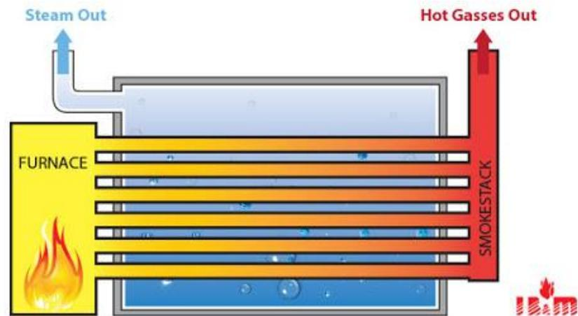
**Gambar 2. 5 Fire Tube Boiler**
