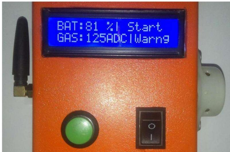
**Gambar 4.19** Tampilan Proses Pendeteksian Kebocoran Gas
